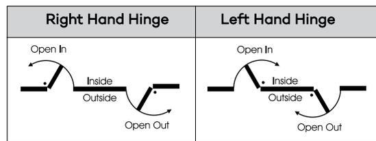
The hand of the hinge must be related to the direction the door opening and the side of the door on which the hinge knuckle is visible. Thus, a left hand door (open in) requires a left hand hinge. However, a left hand hinge is also required for a right hand reverse door (open out). Consequently the opposite applies for a right hand hinge (refer hinge handing above).
